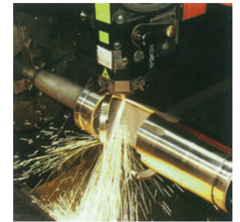
Hunter Innovations uses advanced laser-etching technology to cut passages in stainless steel piping that will accept the backflow-prevention components.
