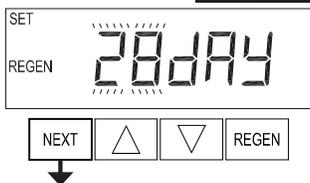
**Step 12S** – Set Regeneration Trigger using ▲ or ▼. If Step 11S is set to OFF, Regeneration Trigger can be set to 28 day or 7 day. Press NEXT to go to Step 13S. Press REGEN to return to previous step.
