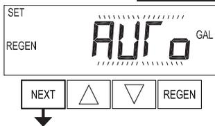
**Step 11S** – Set Volume Capacity using ▲ or ▼. If value is set to:
