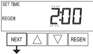
**Step 4I** – Next Regeneration Time (hour): Set the hour of day for regeneration using ▲ or ▼. The default time is 2:00. Press NEXT to go to step5I. Press REGEN to return to previous step.
