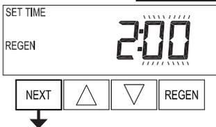
**Step 5I** – Next Regeneration Time (minutes): Set the minutes of day for regeneration using ▲ or ▼. Press NEXT to exit Installer Display Settings. Press REGEN to return to previous step.
